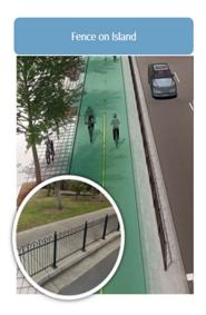
This scenario would construct a concrete median, with the installation of wrought iron fencing that would match the fencing in other downtown locations, such as Children's Park along Esplanade. This provides a physical barrier from adjacent vehicle travel lanes, however lacks landscaping features that typically provide a more welcoming environment.
